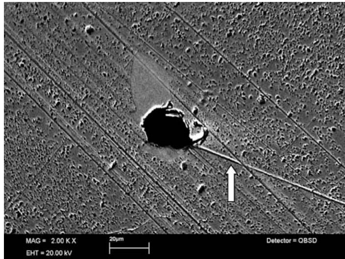
Fig. 6 Partially pulled-out carbide with a scratch (arrow) originating from the defect.
